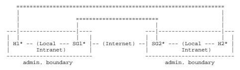
Case 4. This covers the situation where a remote host (H1) uses the Internet to reach an organization's firewall (SG2) and to then gain access to some server or other machine (H2). The remote host could be a mobile host (H1) dialing up to a local PPP/ARA server (not shown) on the Internet and then crossing the Internet to the home organization's firewall (SG2), etc. The
