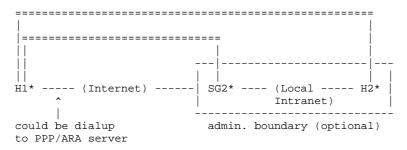
Only tunnel mode is required between H1 and SG2. So the choices for the SA between H1 and SG2 would be one of the ones in case 2. The choices for the SA between H1 and H2 would be one of the ones in case 1.
